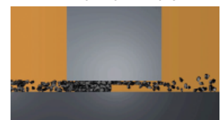
CONTAMINATION IN PRESENCE OF NARROW TOLERANCES
